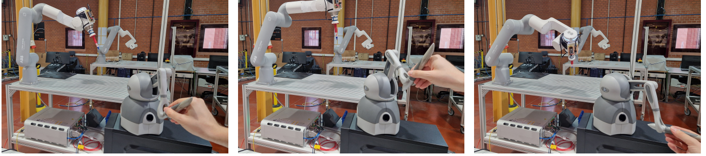
Figure 8: Drawing teleoperation task with ABB GoFa.
