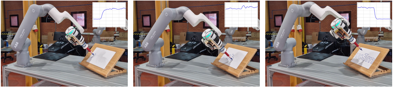
Figure 7: Drawing task with path correction using external force-torque feedback. The normal force component is depicted using the “rqt plot” tool.
