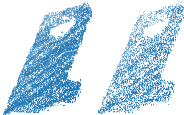
Figure 1: Visual comparison of the 3D point clouds extracted from a physical base plate replica, showing subsampled resolutions of 8192 points (left) and 4096 points (right).
